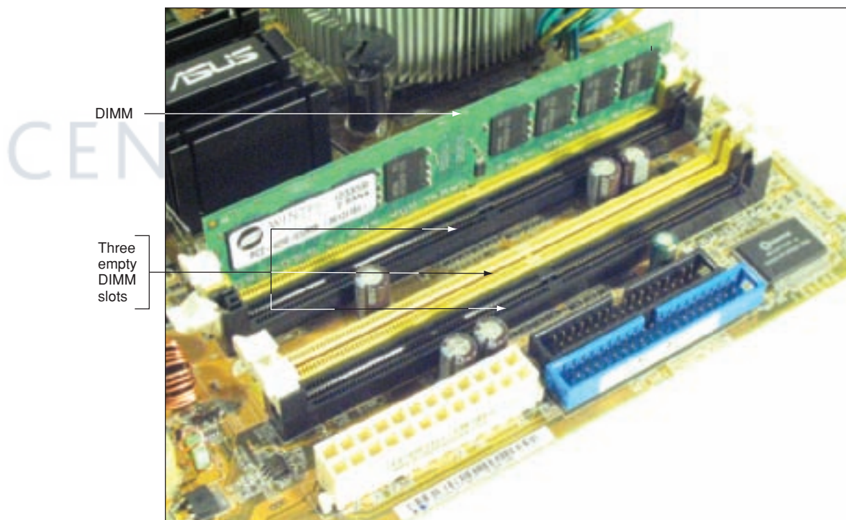
Figure 1-13 A DIMM holds RAM and is mounted directly on a motherboard Courtesy: Course Technology/Cengage Learning
