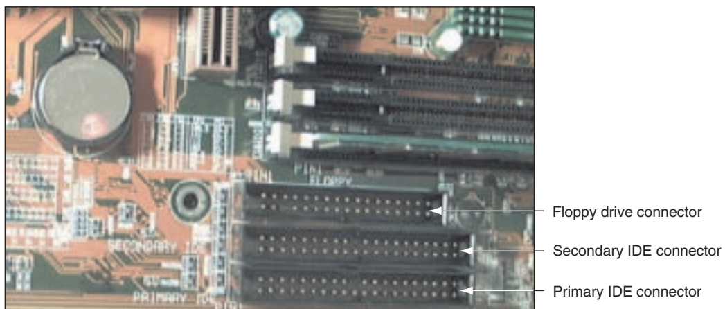
Figure 1-25 A motherboard usually provides a connection for a floppy drive cable Courtesy: Course Technology/Cengage Learning
