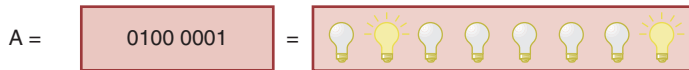
Figure 1-3 All letters and numbers are stored in a computer as a series of bits, each represented in the computer as on or off Courtesy: Course Technology/Cengage Learning
