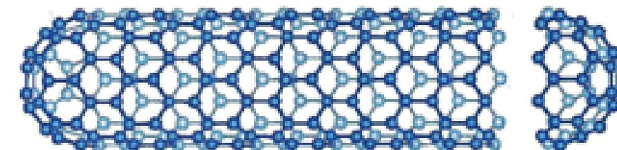
zigzag nanotube  $(n,0)$   $\theta = 0^\circ$
