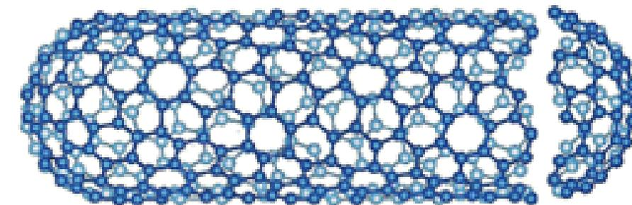
chiral nanotube  $(n,m)$   $0 < \theta < 30^\circ$
